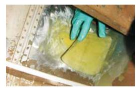
Photo 7—Three layers of glass were laid in position on the inside of the hull and lightly squeegeed to remove trapped air.
